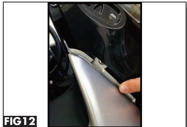
Fig 12. A closer view of the plastic tabs and the slots. (For reference.)
