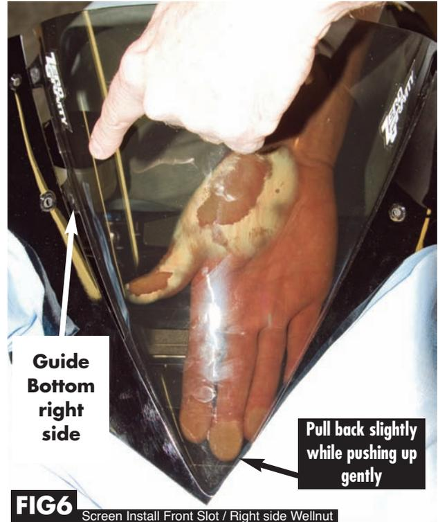
**Fig 6.** Pull back the screen slightly and push up to slide the Tip of the screen into the fairing slot. Once Tip of the screen is inserted and in place, **Apply light pressure** where the finger is pointing to flex the windscreen. Position the bottom right side wellnut in between the fairing and frame.
