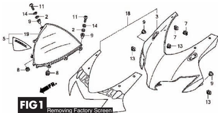
**FIG1** Removing Factory Screen
