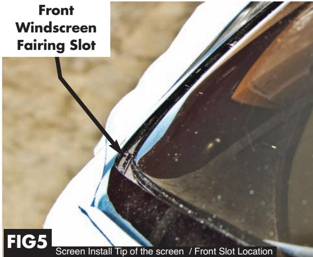
**Fig 5.** Locate front windscreen fairing slot. It should look like this in front of the windscreen.
