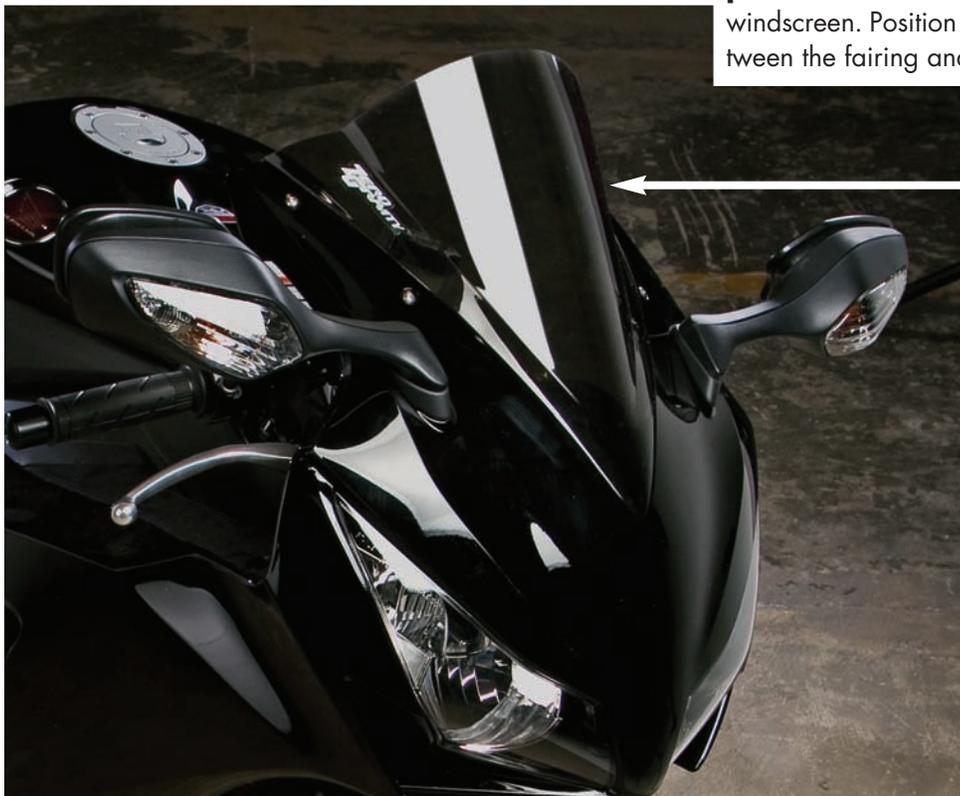
The screen is ready to finish the install, add 4 fasteners to the wellnuts to complete the install.
