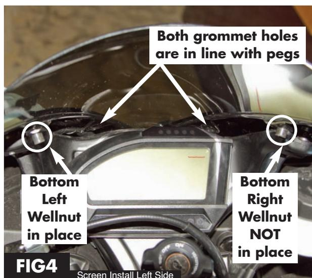
**FIG4** Screen Install Left Side
