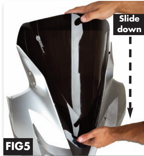
Fig 5. Now you are ready to lock the screen into the fairing. Apply light pressure from the top to slide the windscreen down. The slide is no more than 1/4".
