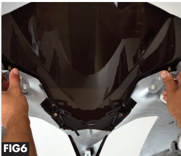
Fig 6. Viewing from the back of the fairing, both fairing stay standoffs should be in alignment with the Zero Gravity windscreen fairing stay standoff openings. See Fig 7 for closeup.
